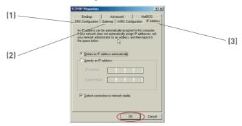
If "Specify and IP address" is selected, your Router will need to be set up for a static IP connection type. Write the address information in the table below. You will need to enter this information into the Router.
